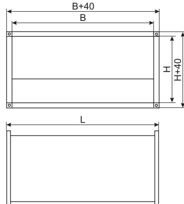
Rectangular duct silencers SKS are designed for rectangular duct fans VKS/VKSA and can be mounted into a system of rectangular air ducts. SKS silencers have good sound attenuation characteristics. Several silencers can be mounted into a rectangular air duct system if there is requirement for bigger noise reduction. The casing is made of galvanized steel and inner casing is made of perforated sheet steel. Rock wool is used for sound insulation.
